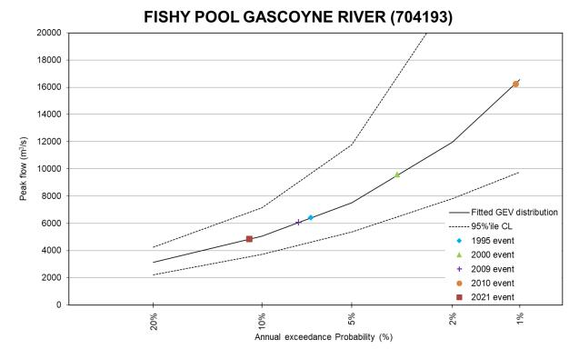
Figure 14 Expected likelihood of the February 2021 event and other recent notable events by peak flow at DWER's Fishy Pool streamflow gauge
