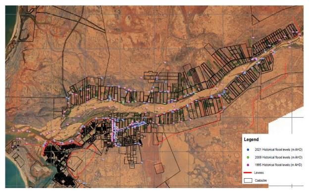
Figure 25 Surveyed peak flood levels for February 2021 and 1995 flood events  $^{\ast}$
