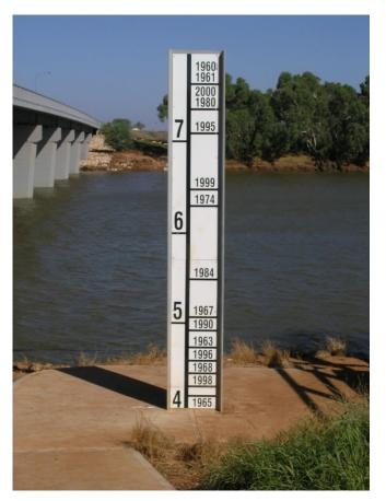
Figure 33 Staff gauge installed downstream of the Nine Mile Bridge
