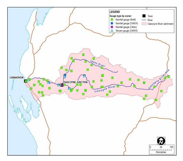
Figure 3 DWER and BoM rainfall gauges within the Gascoyne River catchment
