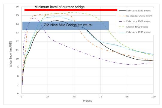
Figure 12 Comparison of recorded water levels at DWER's streamflow gauging station at Nine Mile Bridge\*
