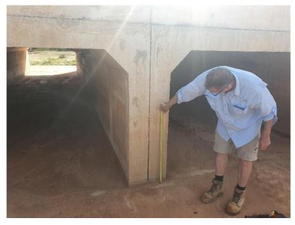
Figure 17 Measuring up from ground to flood mark (downstream side of culverts at Six Mile Creek crossing of North West Coastal Highway)
