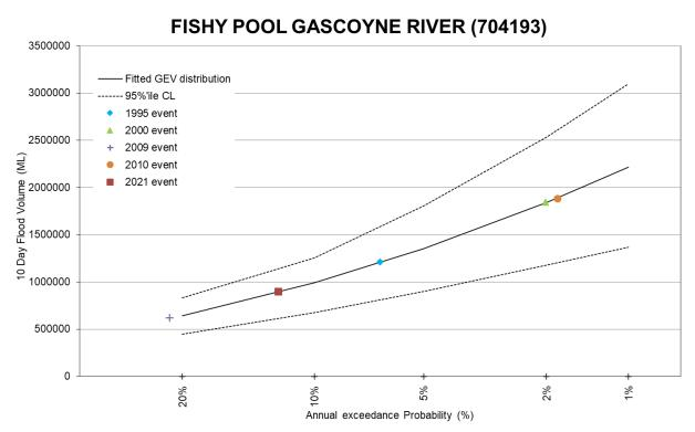
Figure 15 Expected likelihood of the February 2021 flood event and other recent notable events based on flow volume over a ten-day period at our Fishy Pool streamflow gauge
