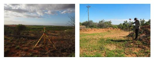
Figure 16 RTK survey (left: base station set up at Landgate survey benchmark, right: rover unit and flood debris mark)
