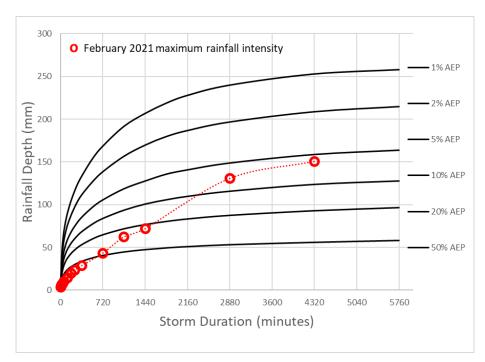
Figure 6 Comparison of February 2021 rainfall intensity at DWER's Fishy Pool rainfall gauge with BoM (2016) design intensity-frequency-duration values
