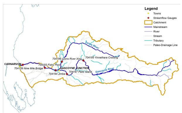
Figure 9 Location of DWER's streamflow gauging stations in the Gascoyne River catchment
