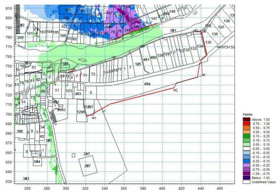
With the private levee incorporated within the hydraulic model, water levels adjacent to SRR are estimated to rise approximately 50 mm compared to modelling without the northern private levee.
