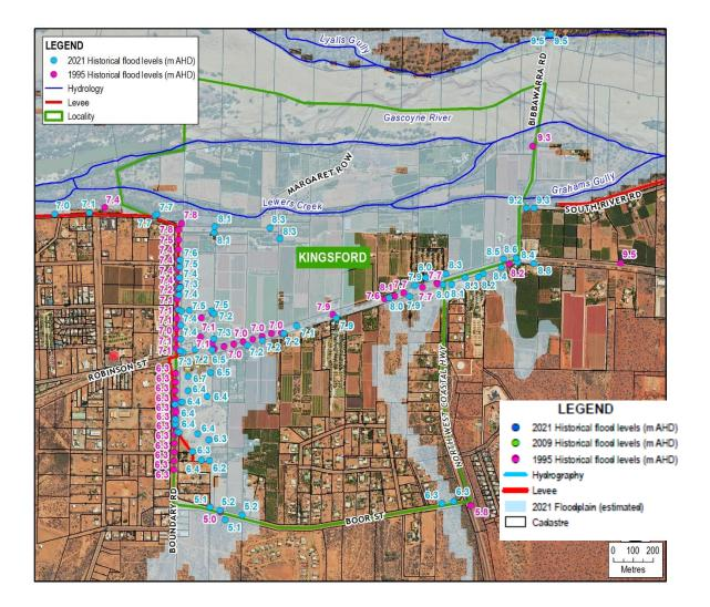
Figure 26 Comparison of 1995 and 2021 surveyed peak water levels in the Kingsford area of Carnarvon
