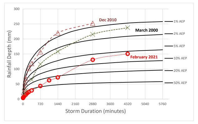
Figure 8 Comparison of the recorded rainfall intensities at DWER's Fishy Pool rain gauge for events in March 2000, December 2010 and February 2021 with BoM (2016) IFD estimates
